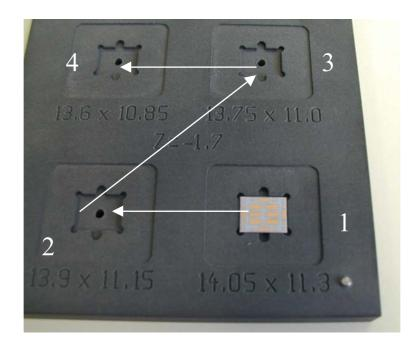
2 Once the best fit location has been found, leave the PA there and put stencil on top of the jig and PA.
